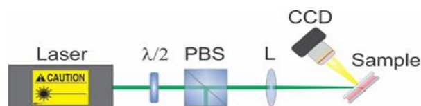
Fig. 2. Scheme of the experimental set-up with pump laser (532 nm , 300 ps and 7 ns pulse width); \lambda/2 (half wave plate for 532 nm ); PBS (polarizing beam splitter); L (lens with 100 mm focal length); CCD (CCD camera).
