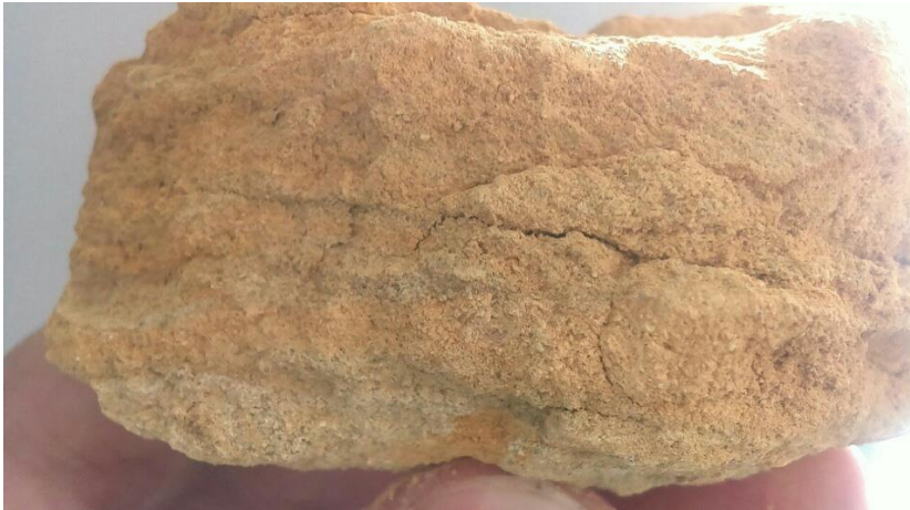
Fig. Waterproofing layer change as a result of geochemical migration
