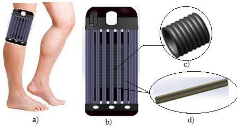
Fig. 4. a) Application of orthosis, b) orthosis, c) flexible joint, d) actuator
