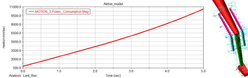
Fig. 5. Power consumption of actuators without considering the flexibility
