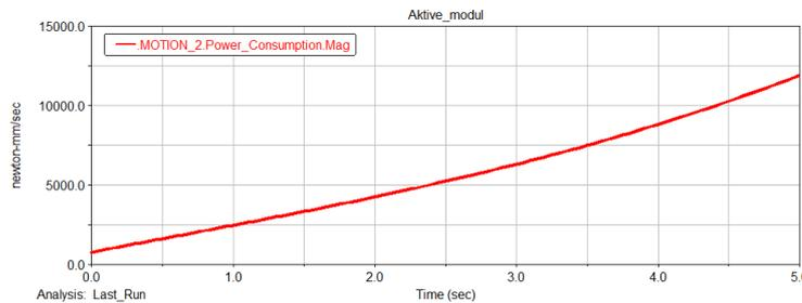
Fig. 6. Power consumption of actuators with considering the flexibility
