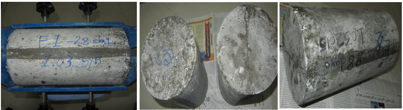
Fig.3. Examine compressive and tensile strength, a hydraulic jack
