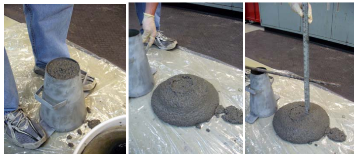
Figure 3: Filling the slump cone, cone removal, measurement of polymer concrete slump
