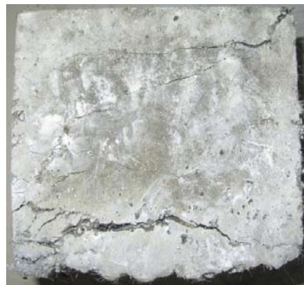
Fig. 7. Failure of high strength concrete with fibers
