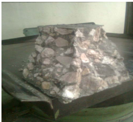
Fig. 6. Failure of high strength concrete with no fibers
