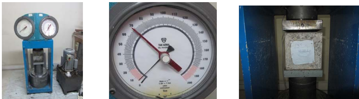
Figure 4: Examine compressive and tensile strength, a hydraulic jack
